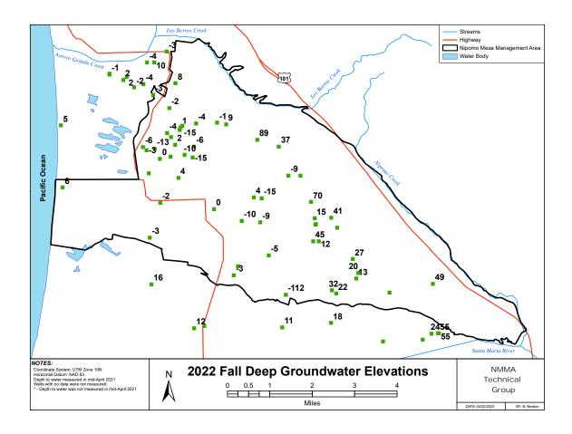
Figure 3-4. 2022 Fall Deep Aquifer Groundwater Elevations
