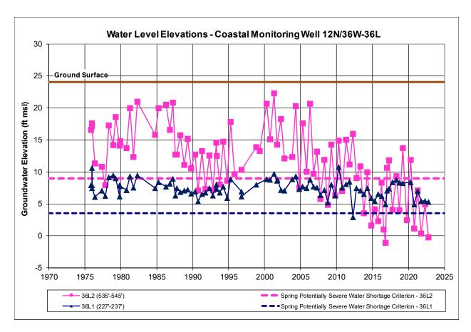
Figure 6-4. Hydrograph for Coastal Monitoring Well Nest 12N/36W-36L
