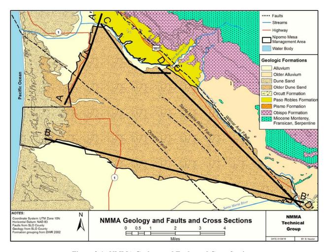
Figure 2-1. NMMA Geology and Faults and Cross Sections
