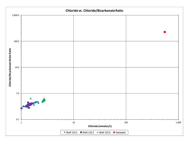
Figure 6-11. Chloride vs Chloride/Bicarbonate Ratio for Coastal Wells
