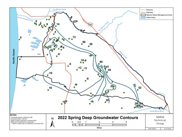
Figure 6-6. 2022 Spring Deep Aquifer Groundwater Contours
