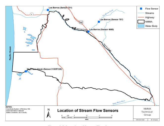
Figure 3-8. Location of Stream Flow Sensors
