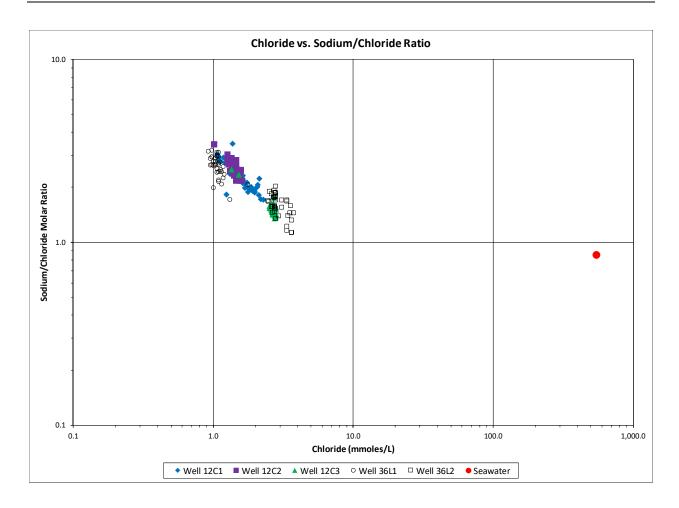
Figure 6-12. Chloride vs Sodium/Chloride Ratio for Coastal Wells
