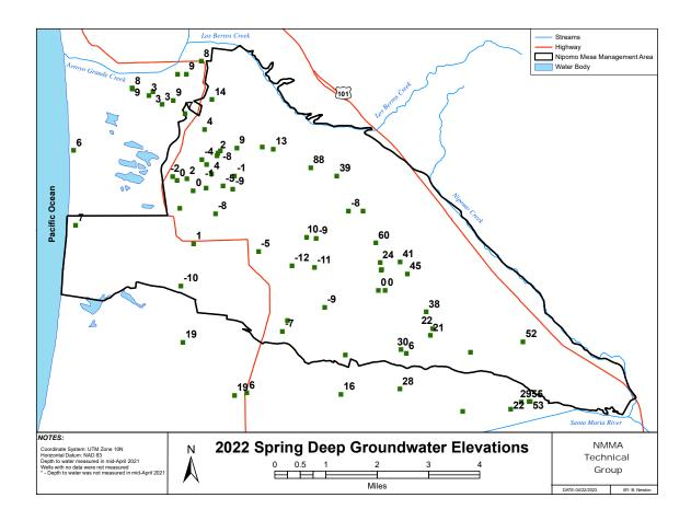
Figure 3-2. 2022 Spring Deep Aquifer Groundwater Elevations
