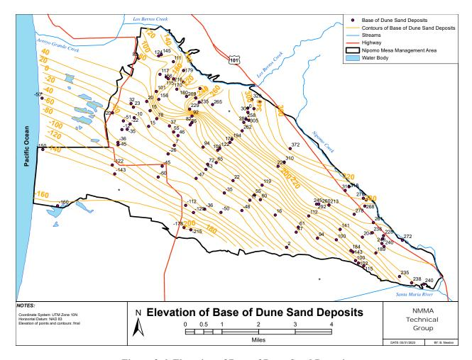
Figure 2-6. Elevation of Base of Dune Sand Deposits
