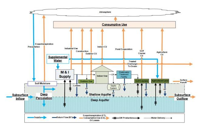
Figure 5-1. Schematic of the Hydrologic Inventory
