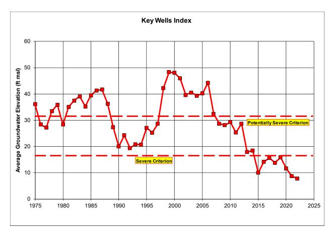
**Figure 7-1. Key Wells Index** *The upper dashed line is the criterion for Potentially Severe Water Shortage Conditions and the lower dashed line is the criterion for Severe Water Shortage Conditions.*
