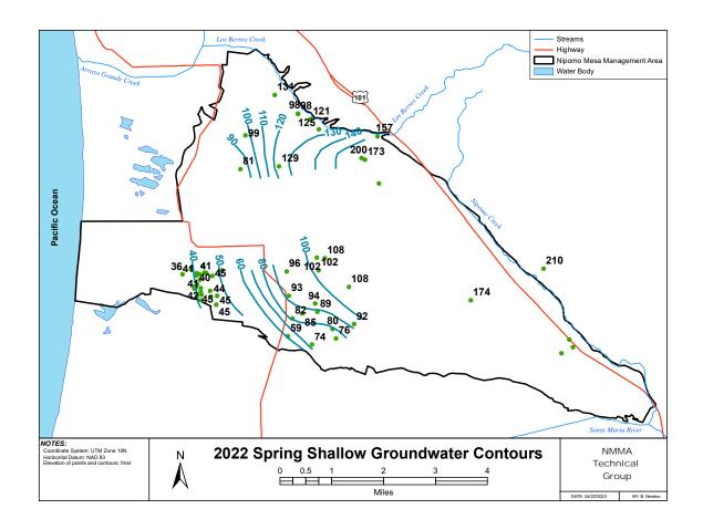
Figure 6-5. 2022 Spring Shallow Aquifer Groundwater Contours
