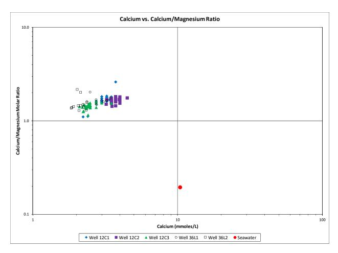
Figure 6-13. Calcium vs Calcium/Magnesium Ratio for Coastal Wells
