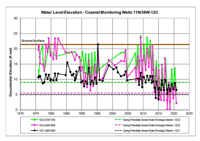
**Figure 6-3. Hydrograph for Coastal Monitoring Well Nest 11N/36W-12**C Note: Water levels measured under artesian flow prior to 2008 were observed without measuring the hydraulic head and recorded as a default value of 2 feet above the casing.
