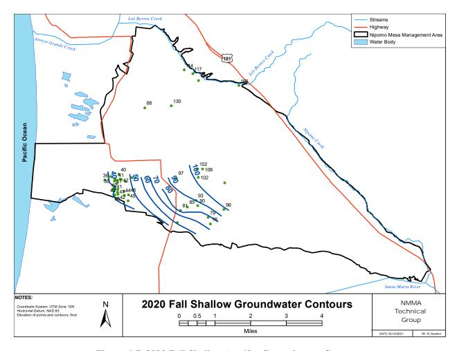
Figure 6-7. 2020 Fall Shallow Aquifer Groundwater Contours
