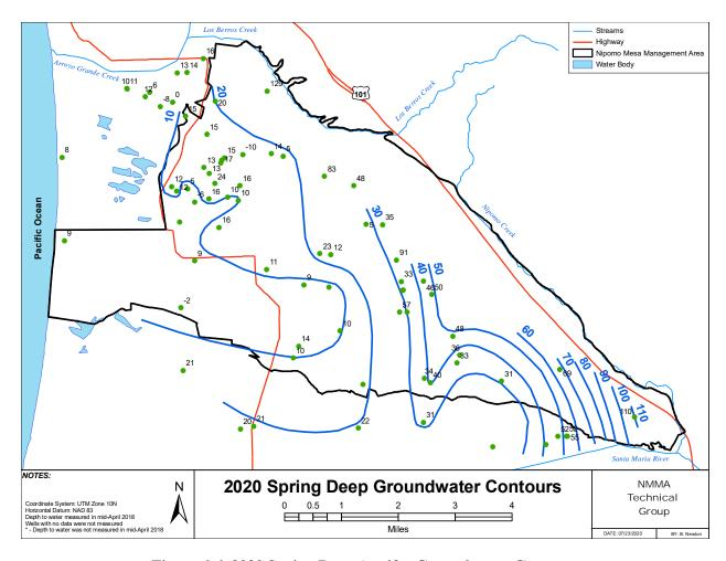
Figure 6-6. 2020 Spring Deep Aquifer Groundwater Contours
