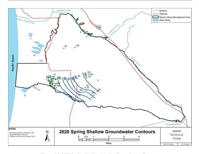
Figure 6-5. 2020 Spring Shallow Aquifer Groundwater Contours
