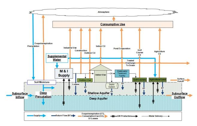
Figure 5-1. Schematic of the Hydrologic Inventory
